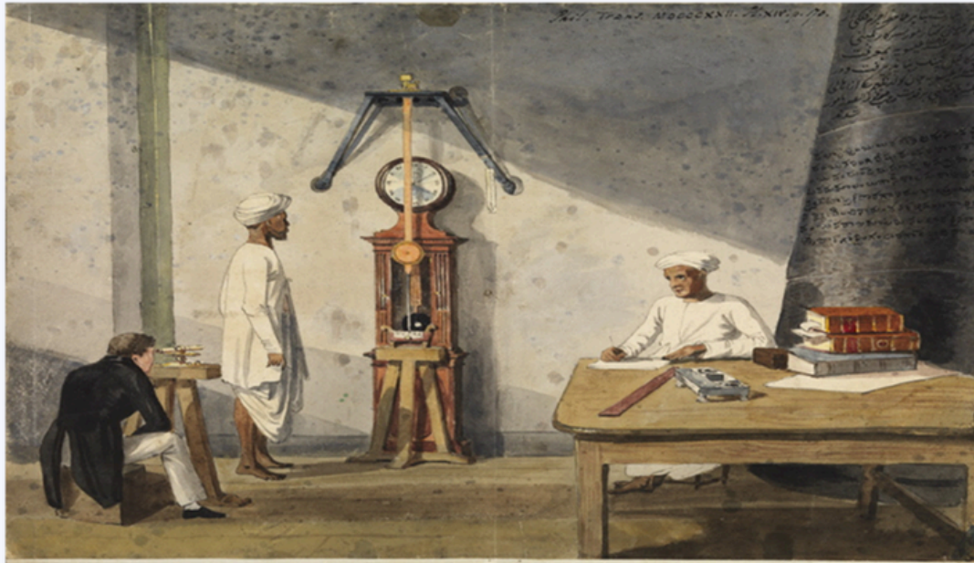
Illustration of the measurement of the acceleration of gravity with an invariable pendulum in Madras by John Goldingham, 1821
